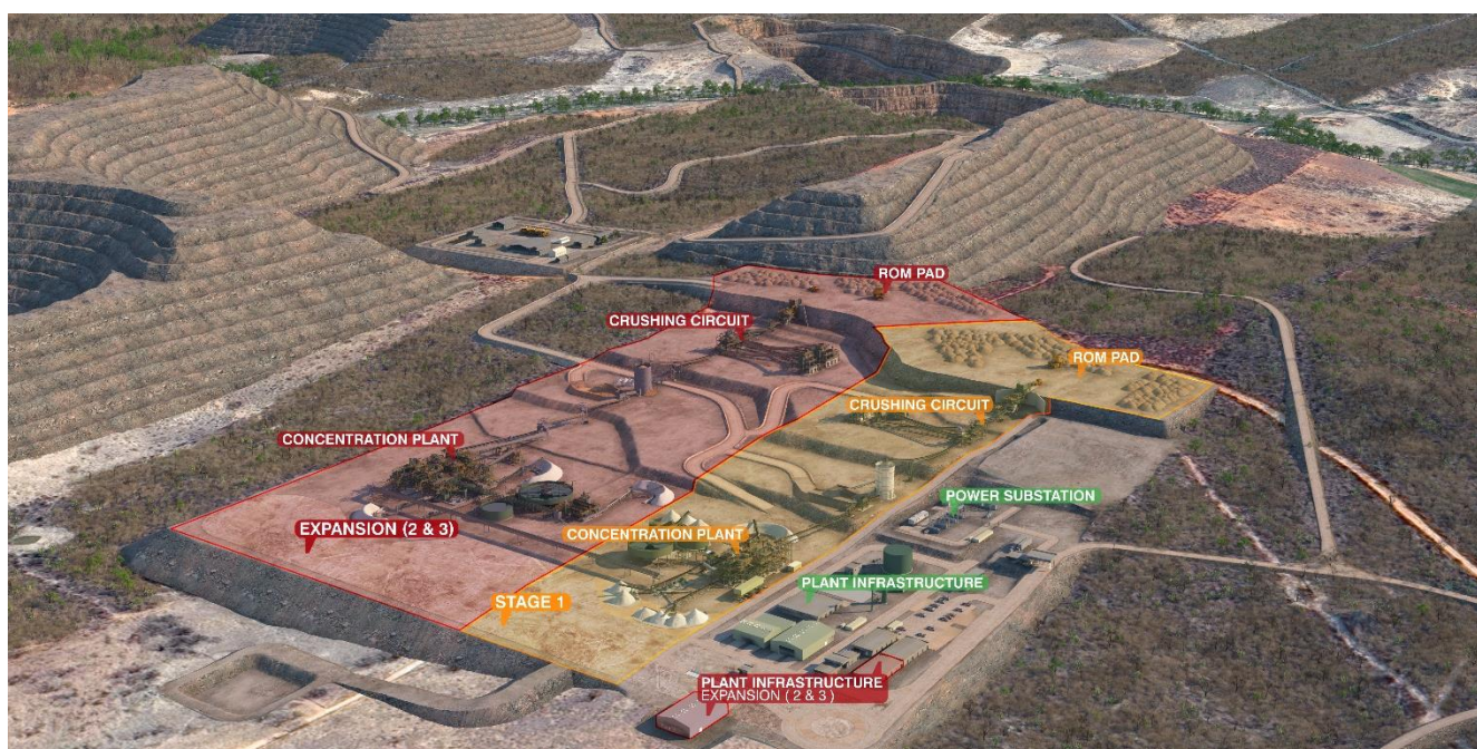
Figure 13: 3D Rendering of the Phase 1 and Potential Phase 2 & 3 Greentech Plant Expansion
